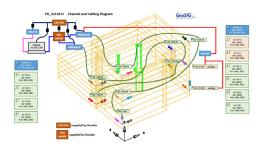
The accelerometers and digital seismic recorders are strategically placed. GeoSMART software monitors the data received from the sensors and sends an alert if exceedances are detected.
